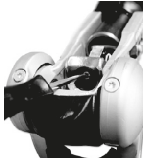
Figure 19 Remove head cap screw
