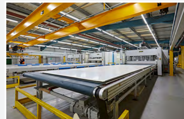
'SMART' GRP sidewall during the production process.
