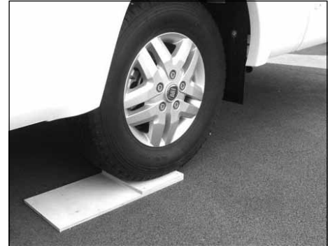
Fig. B Stepped levelling board
