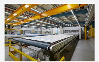
'SMART' GRP sidewall during the production process.
