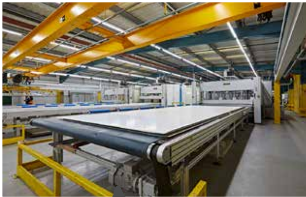
'SMART' GRP sidewall during the production process.
