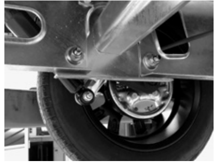
Fig. C - Reinforced axle plate
