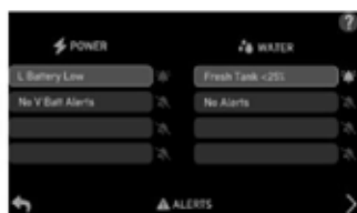
Example Power / Water warnings
