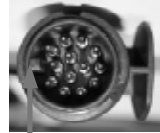
Incorrect alignment Fig. 7
